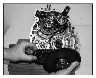
8. Remove roller chain. Note position of sprockets and gear. Stretch chain tight on a flat surface and measure the length of 8 pitches in a minimum of three places on chain. Replace chain if measurement is longer than 5.05 (128.27 mm).
