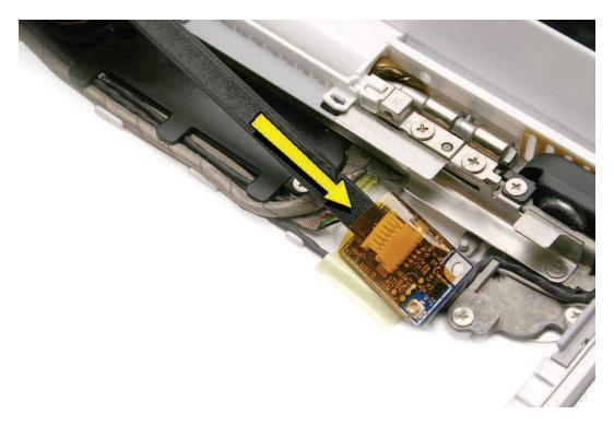
Replacement Note: Connect the Bluetooth-to-logic board cable first before adhering the board to the bottom case. Then install the Bluetooth antenna cable, and make sure the cable exits toward the upper right corner of the bottom case.
