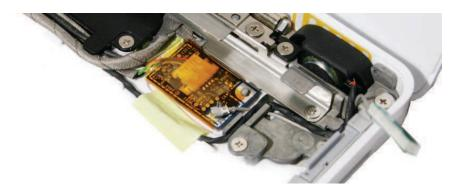
**Replacement Note:** Make sure the upper right corner of the board fits over the locator pin. To secure the board, press only the right corners of the board near the locator pin and the Bluetooth antenna cable.
