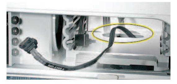
Then install the lower hard drive with the cable routed above the drive, and connect the cable to the drive as illustrated.
