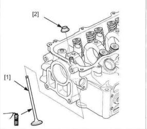
Apply engine oil to the inner wall of a new valve stem seal [1].
